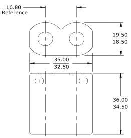
This battery contains a Positive Temperature Coefficient (PTC) safety device to limit current during short circuit conditions.
